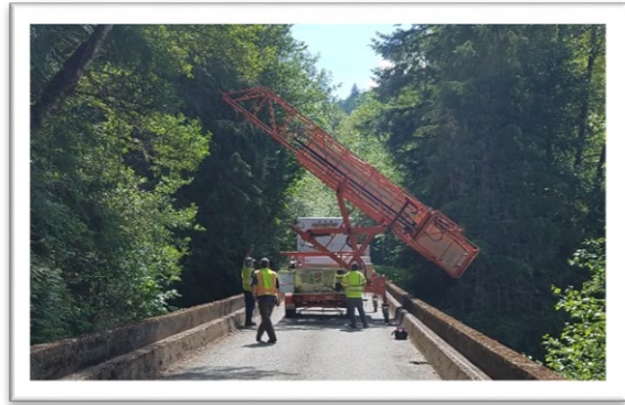
Whatcom Co Hydro-Platform on Finney Cr Bridge
